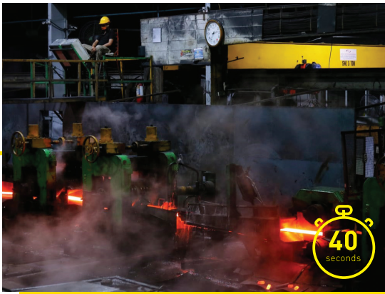
PLC CONTROLLED CONTINUOUS LINEAR ROLLING MILL TO ENHANCE PRODUCTION SPEED - 30 METRES PER SECOND WHILE PROCESSING IN 23 PASSES
