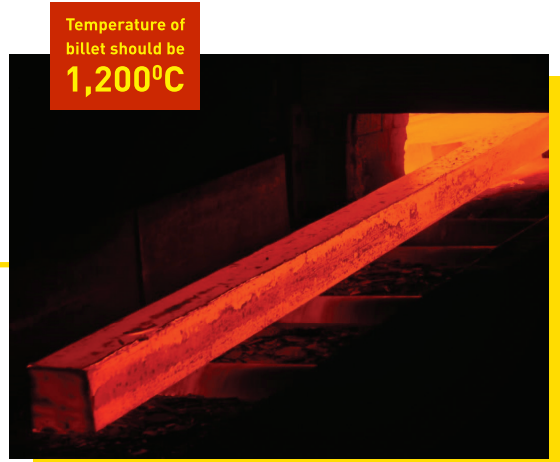
SOUTH INDIA'S FIRST FULLY AUTOMATED FURNACE TO MAINTAIN THE TEMPERATURE OF THE BILLET AT 1,200° C
