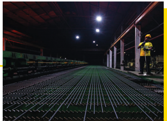
AUTOMATED HIGH-SPEED COOLING BED TO ENSURE SUPERIOR-QUALITY TMT BAR
